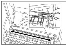
Run the brush from side to side along the separator as shown to remove any soiling.
